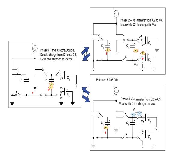
Figure 1. Charge pump phases
