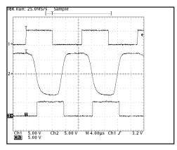
Figure 4, Loopback results at 60KHZ and 2500pF load (1 = TXin, 2 = TXout/RXin, 3 = RXout).
