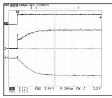
Figure 5, Charge pump outputs at start up (1 = Vcc, 2 = V+, 3 = V-).
