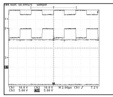
Figure 2, SP233A Charge pump waveformsno load (1 = C1+, 2 = C2+, 3 = V+, 4 = V-).
