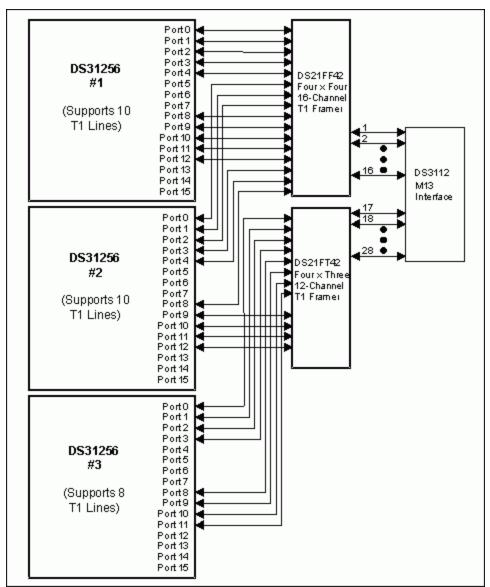
Figure 7. Single T3 with 672 HDLC channel support.
