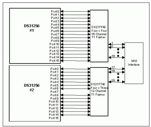
Figure 6. Single T3 with 512 HDLC channel support.
