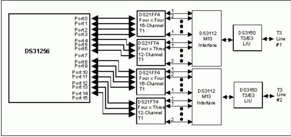
Figure 5. Dual T3 with 256 HDLC channel support.
