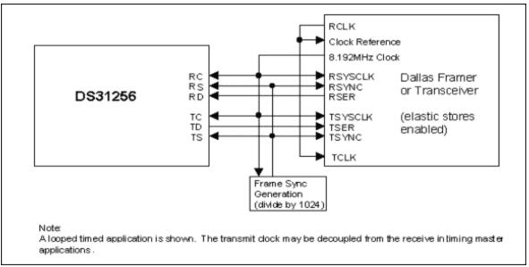
Figure 3. Quad T1/E1 connection.
