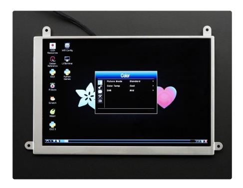
Picture Mode - Bright, Standard, Soft, user Color Temp - Warm, Normal, Cool, User DNR (Digital Noise Reduction) - Off, Low, Medium, High
