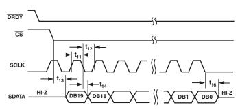
Figure 5a. SEC Mode Timing Diagram
