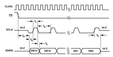
Figure 6. SSC Mode Timing Diagram
