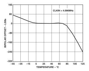
Figure 13. Typical Bipolar Offset vs. Temperature after Calibration at 25°C
