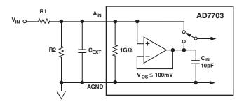
Figure 14. Equivalent Input Circuit and Input Attenuator
