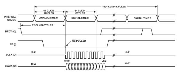
Figure 15. Timing Diagram for SSC Transmission Mode
