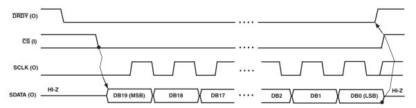
Figure 17. Timing Diagram for SEC Mode
