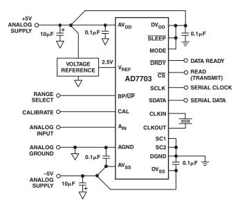
Figure 7. Typical System Connection Diagram
