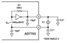
Figure 11. On-Chip Gate Oscillator
