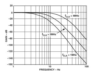
Figure 9. Frequency Response of AD7703 Filter
