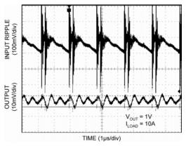
Figure 11. Ripple Reduction
