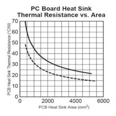
Figure 8. PC Board Heat Sink
