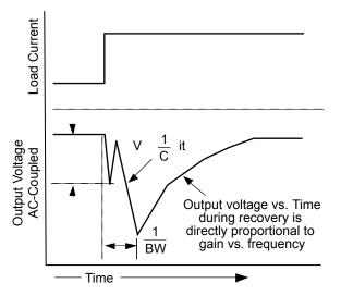
Figure 2. Typical Transient Response
