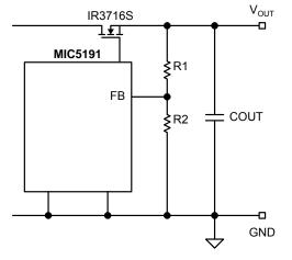
Figure 10. Adjustable Output
