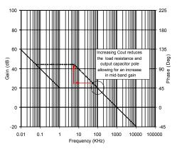
Figure 7. Increasing Output Capacitance
