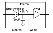
Figure 3. Internal Compensation
