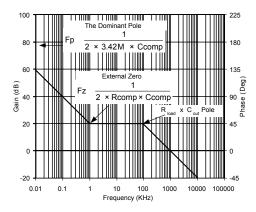
Figure 6. External Compensation Frequency Response
