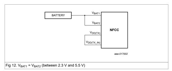
$V_{DD(TX)}$  value shall be chosen according to the minimum targeted  $V_{BAT}$  value for which reader mode shall work.
