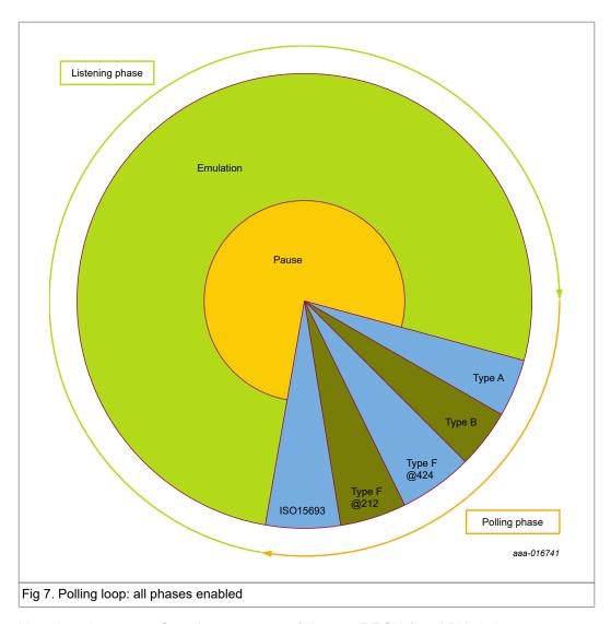
Listening phase uses Standby power state (when no RF field) and PN7150 goes to Listener mode when RF field is detected. When in Polling phase, PN7150 goes to Poller mode.
