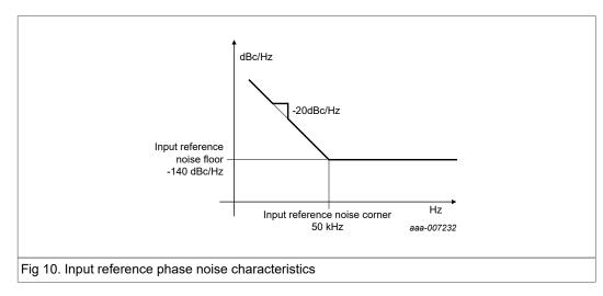
This phase noise is equivalent to an RMS jitter of 6.23 ps from 10 Hz to 1 MHz. For configuration of input frequency, refer to [9]. There are 6 pre-programmed and validated frequencies for the PLL: 13 MHz, 19.2 MHz, 24 MHz, 26 MHz, 38.4 MHz and 52 MHz.
