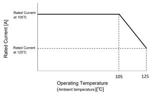
• Operating Temperature : - 40 °C to + 125 °C Storage Temperature : -40 °C to + 125 °C
