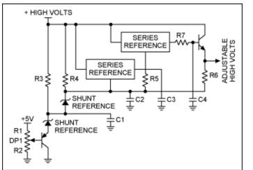
Figure 3. The high voltage applied is limited by the sum of the stacked references.
