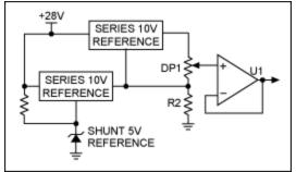
Figure 2. This design also features the MAX5437/MAX5439 digital pots, but here the voltage is independent of the pot's end-to-end resistance and tolerance.
