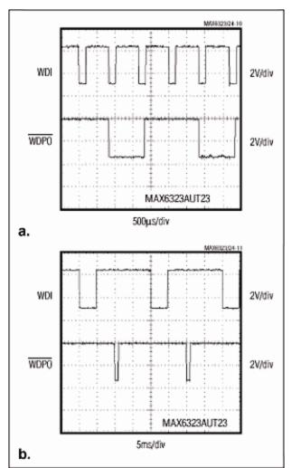
Figure 4. These actual waveforms illustrate fast (a) and slow (b) timeout faults.
