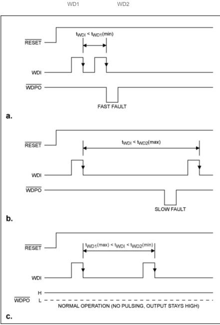
Figure 1. These timing diagrams illustrate fast (a) and slow (b) watchdog-timing faults.
