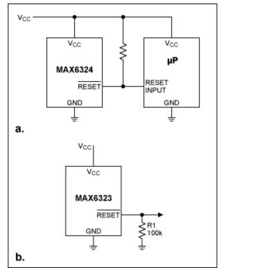
Figure 2. Output stage connections: open-drain MAX6324 (a), and push-pull MAX6323 (b).
