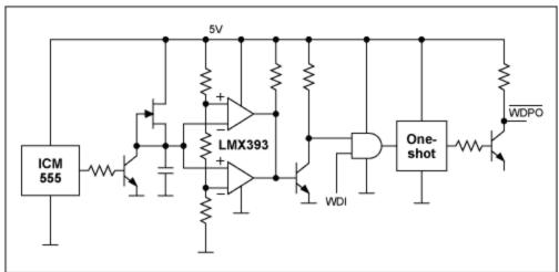
Figure 5. Discrete-component example of a windowed-watchdog timer.
