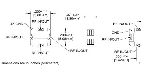
Dimensions are in Inches [Millimeters] X2B Rev A Mechanical Outline
