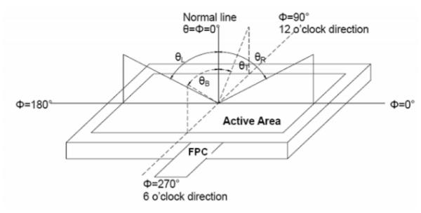
FIG. 3 The definition of Viewing Angle
