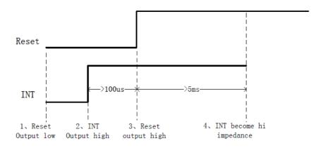
Fig.8(a) Timing of setting slave address
