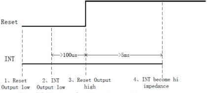
Fig.8(b) Timing of setting slave address
