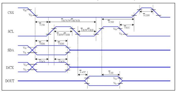
Figure 5 4-line serial Interface Timing Characteristics
