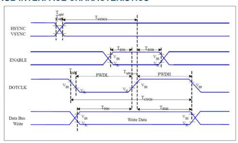
Figure 6 RGB Interface Timing Characteristics
