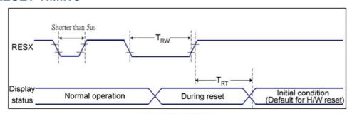
Figure 7 Reset Timing
