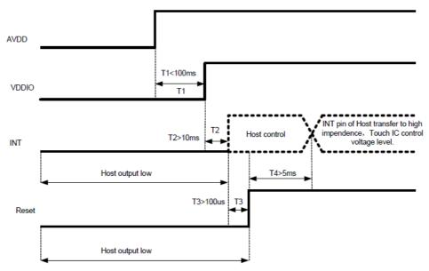
Fig.7 Power on diagram
