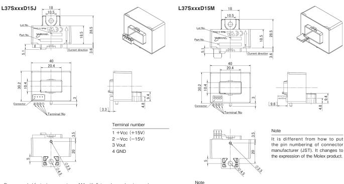
· Recommended fastening screw type : M4 with flat washer and spring washer  $\cdot$  Recommended fastening torque : < 1.5 N  $\cdot$  m
