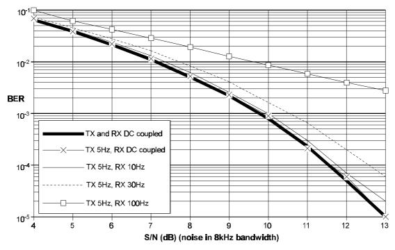
Figure 13: Effect of AC Coupling on Typical Bit-Error Rate
