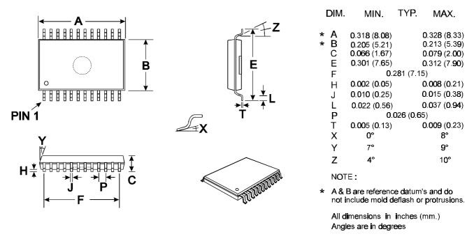
Figure 16: 24-pin SSOP Mechanical Outline: Order as part no. CMX589AD5
