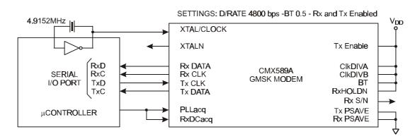
Figure 4: Minimum mController System Connections
