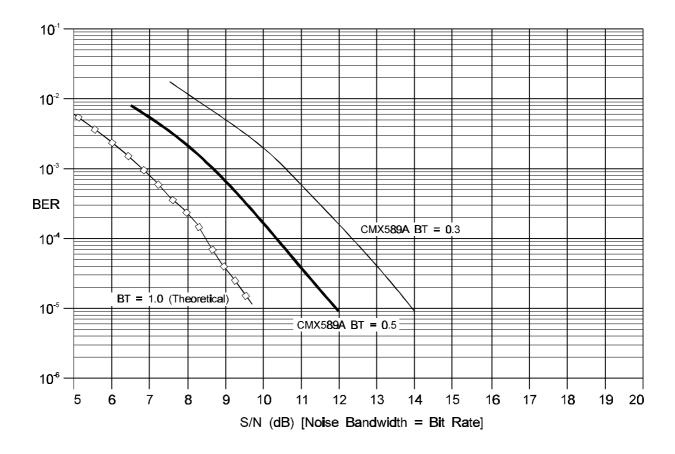
Figure 6: Typical Bit-Error-Rate Performance at V<sub>DD</sub> = 5.0V
