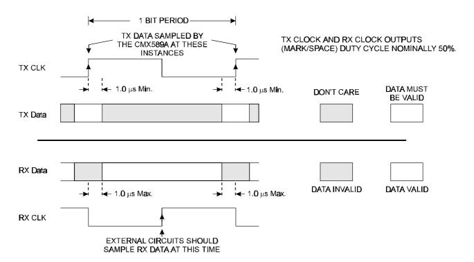
Figure 8: Rx and Tx Clock Data Timings
