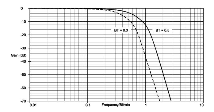
Figure 9: Tx Filter Response
