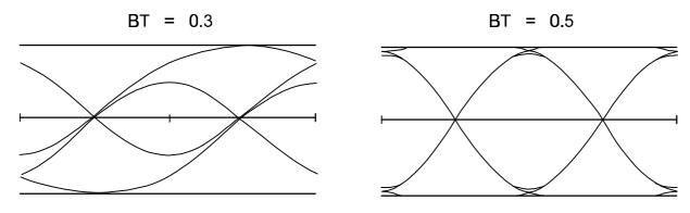
Figure 10: Typical Transmit Eye Patterns
