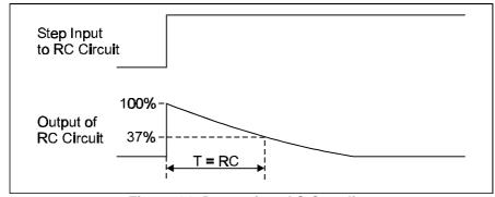
Figure 14: Decay time-AC Coupling
