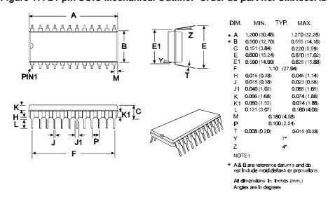
Figure 18: 24-pin PDIP Mechanical Outline: Order as part no. CMX589AP4
