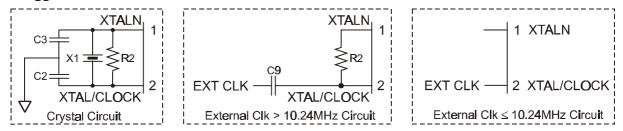
Figure 3: Recommended External Components
