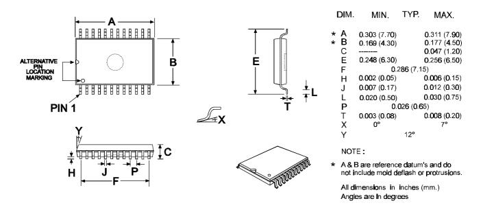
Figure 15: 24-pin TSSOP Mechanical Outline: Order as part no. CMX589AE2
