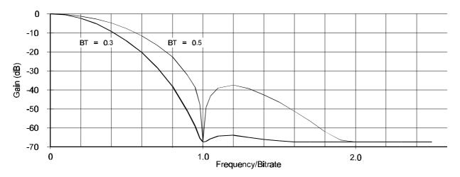
Figure 11: Tx Output Spectrum (Random Data)
