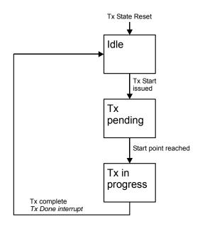
Figure 9 Tx (DSC mode) state transitions
