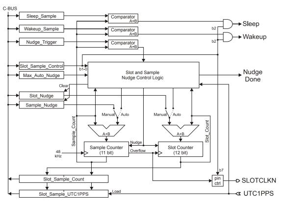
Figure 5 Slot and Sample Timer Circuit
