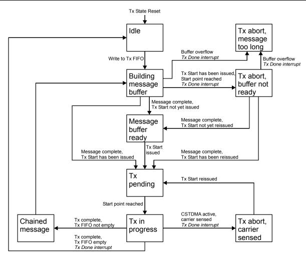
Figure 8 Tx (AIS burst mode) state transitions
