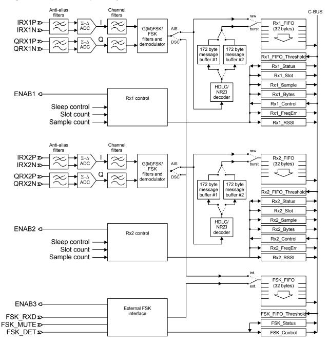
Figure 11 Receive Channel
