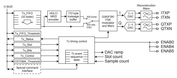
Figure 6 Transmit Channel
