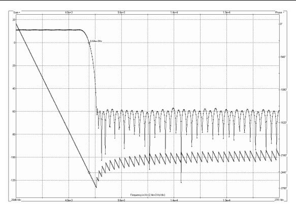
Figure 15 I/Q Filter response in 25kHz operation.
