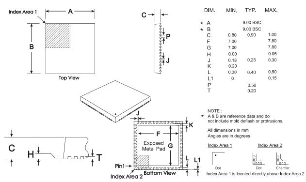
Depending on the method of lead termination at the edge of the package, pull back (L1) may be present. L minus L1 to be equal to, or greater than 0.3mm
