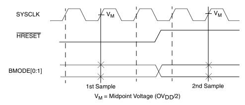
Figure 5. BMODE[0:1] Input Sample Timing Diagram
