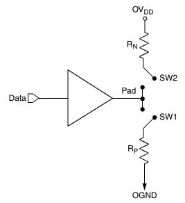
Figure 20. Driver Impedance Measurement
