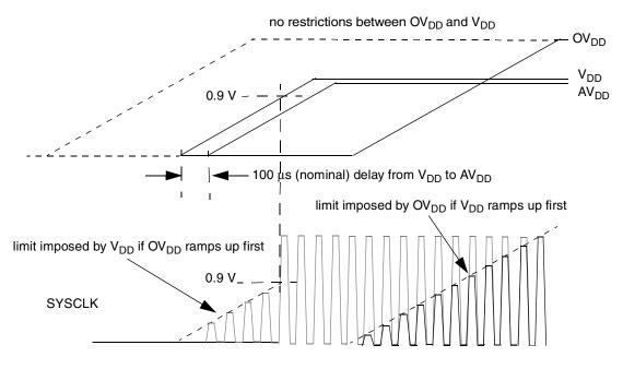
Figure 16. MPC7448 Power Up Sequencing Requirements
