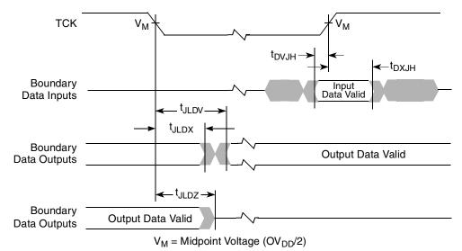
Figure 10. Boundary-Scan Timing Diagram
