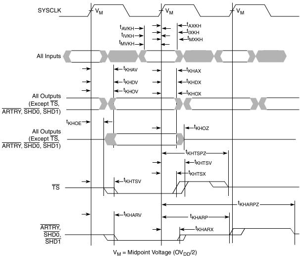
Figure 6. Input/Output Timing Diagram
