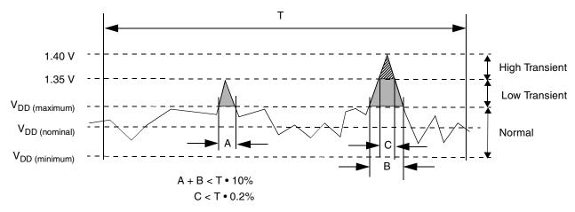
Figure 19. Voltage Transient Example
