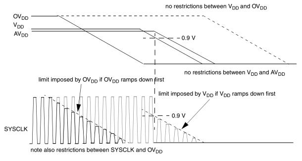
Figure 17. MPC7448 Power Down Sequencing Requirements
