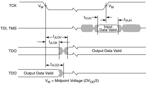
Figure 11. Test Access Port Timing Diagram
