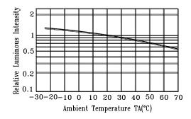
Fig.5 Luminous Intensity vs.
