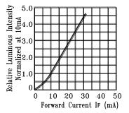
Fig.4 Relative Luminous Intensity vs. Forward Current
