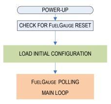
Figure 1. MAX17055 fuel gauge model loading sequence.
