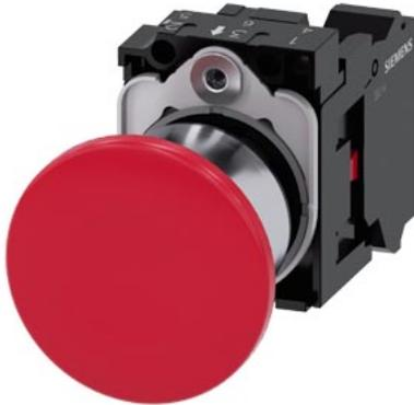
Mushroom pushbutton, 22 mm, round, metal, shiny, red, 40mm, latching, pull-to-unlatch mechanism, with holder, 1 NC, spring-type terminal, with laser labeling, inscription or symbol Customer-specific selection with SIRIUS ACT configurator (CIN)
