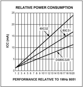
Figure 2. Reduced clock cycle core uses less current for same throughout.
