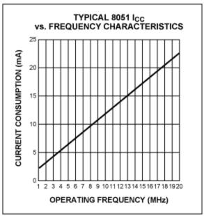
Figure 1. Typical power curve for generic 8051 microcontroller.
