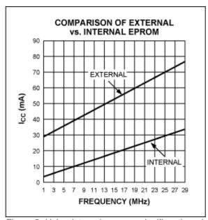
Figure 3. Using internal memory significantly reduces current consumption.
