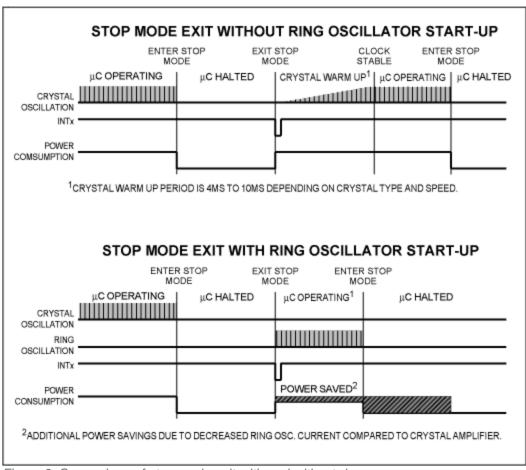
Figure 6. Comparison of stop mode exit with and without ring.
