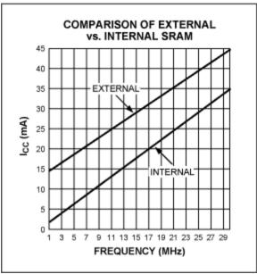
Figure 4. Eliminating external SRAM and latch saves power.
