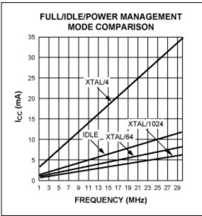
Figure 7. Full/Idle/Power Management Mode Comparison.
