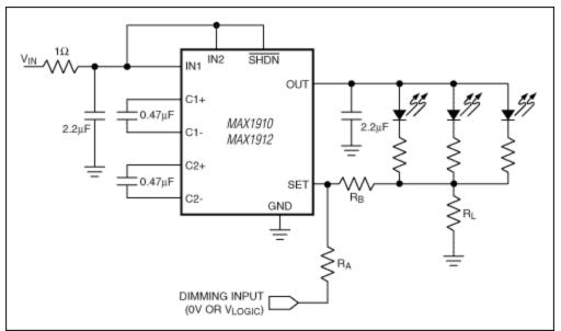
Figure 12. MAX1910/MAX1912 application with a dimming control.
