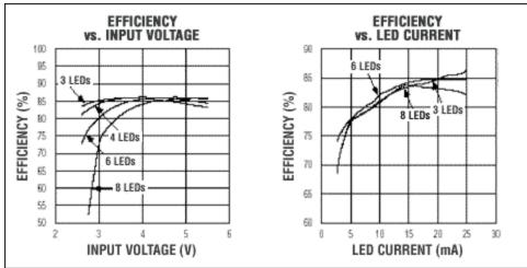
Figure 14. MAX8596Z efficiency for the circuit of Figure 13.
