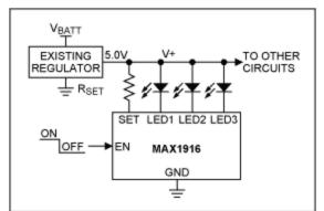
Figure 4. The MAX1916 is available in a SOT23 package and provides 0.3% current matching.
