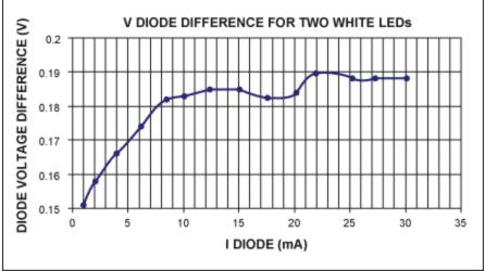
Figure 9B. The voltage difference between two white LEDs vs. current.
