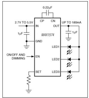
Figure 6. MAX1574 charge pump with one group of LED current sources.
