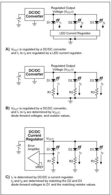
Figure 3. Three methods of driving parallel LEDs are shown. A) Independently regulates the current through each LED. B) Regulates the output voltage and relies on series resistors to match currents. C) Regulates the current in one LED and relies on series resistors to match the remaining currents.
