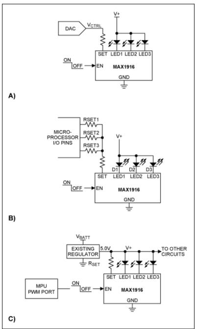
Figure 5. Three methods for adjusting the current in white LEDs with a MAX1916.
