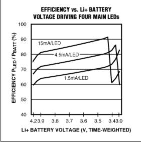
Figure 8. MAX1576 efficiency at typical lithium battery voltages.
