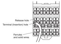
If a wire is difficult to connect because it is too thin, use a flat-blade screwdriver in the same way as when connecting stranded wire.
