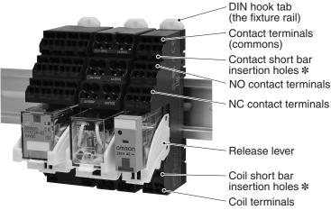
\* The PTF-□□-PU Sockets do not have short bar insertion holes.
