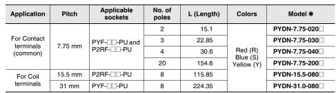
Note: 1. Use the Short Bars for crossover wiring within one Socket or between Sockets.
