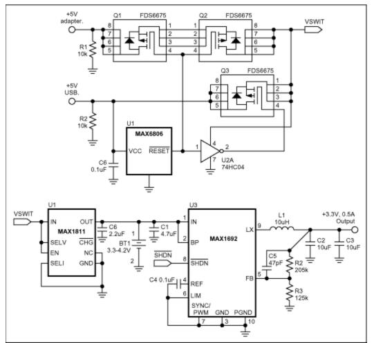
Figure 2. To retain the advantage of seamless switching while eliminating the possibility of connecting both supplies at once, substitute a MOSFET for the diode in Figure 1 and add a voltage detector (U1) and inverter (U2). The resulting circuit allows the designer to set a precise switchover point.
