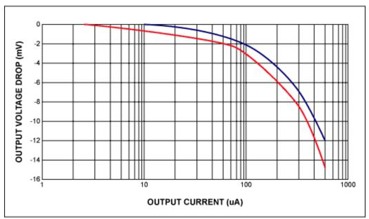
Figure 2. The load-regulation error of the circuit's output.
