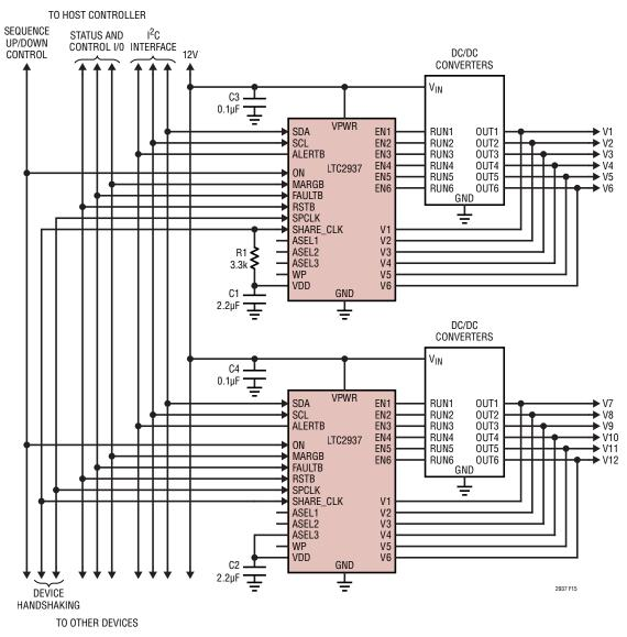
Figure 15. Typical Connections Between Multiple LTC2937s
