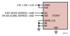
Figure 14. Programming Socket Connections
