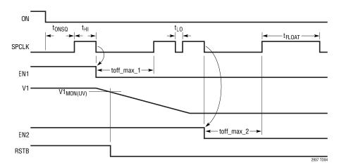
Sequencing 2 Channels (V1, V2), Both Combined into RSTB Logic. toff\_max Timers Used for Post Disable Sequencing Delay; ON\_OFF\_CONTROL b[0] = 1
