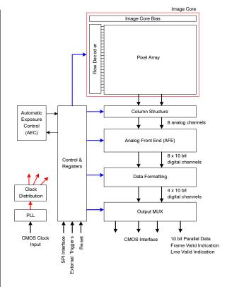
Figure 10. Block Diagram - P2-SN/SE
