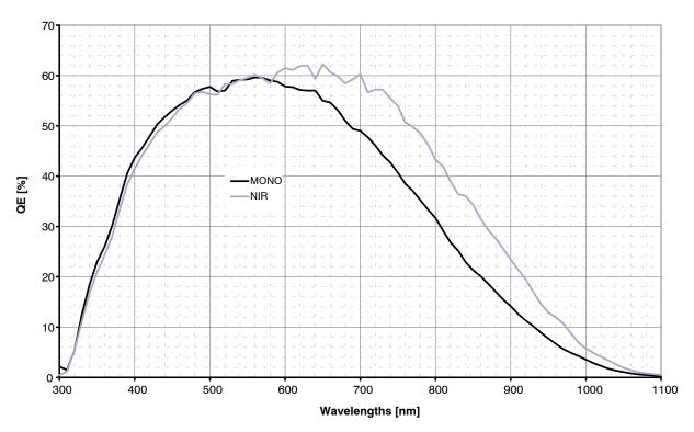
Figure 4. Quantum Efficiency Curve for Standard and NIR Mono
