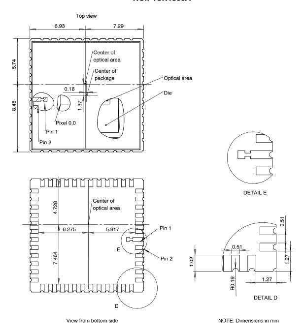
Figure 52. Graphical Representation of the Optical Center (2 of 2)
