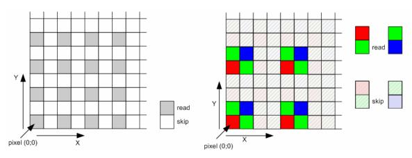
Figure 29. Subsampling Scheme for Monochrome and Color Sensors
