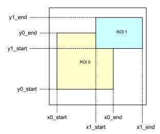
Figure 27. Overlapping Multiple Window Configuration
