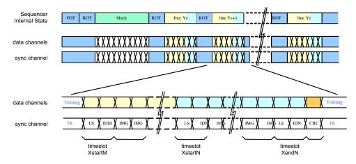
Figure 34. P1-SN/SE/FN, P3-SN/SE/FN: Time Line Showing the Readout of Two Overlapping Windows
