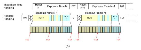
Figure 31. P1-SN/SE/FN, P3-SN/SE/FN: Frame Sync Codes
