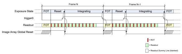
Figure 25. Exposure Time Control in Global-Slave Mode
