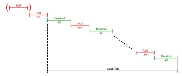
Figure 15. Integration and Readout Sequence of the Sensor Operating in Pipelined Global Shutter Mode with Normal ROT Readout.
