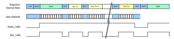
Figure 45. P2-SN/SE/FN: Frame Timing Indication
