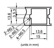
Figure 56. Dimensions of the Protective Foil
