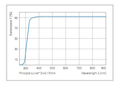
Figure 55. Transmission Characteristics of the Glass Lid
