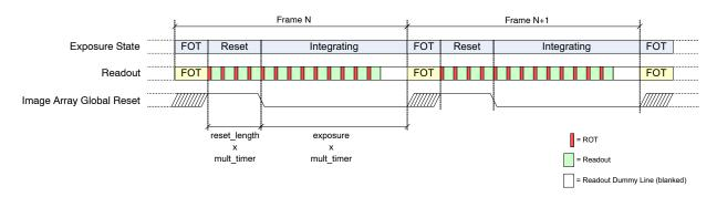
Figure 23. Integration Control for (Pipelined) Global Shutter Mode (Master)
