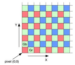
Figure 2. Color Filter Array for the Pixel Array
