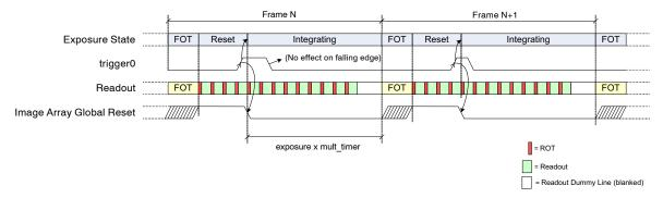
Figure 24. Exposure Time Control in Triggered Shutter Mode (Master)
