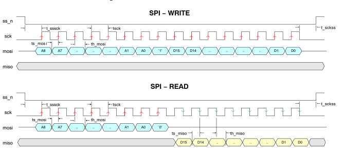
Figure 22. SPI Read and Write Timing Diagram
