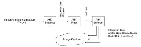
Figure 30. Automatic Exposure Control Loop
