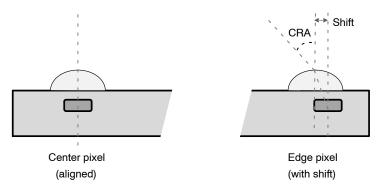
The center axes of the microlens and the photodiode coincide for the center pixels. For the edge pixels, there is a shift between the axes of the microlens and the photodiode causing a Peak Response Incidence Angle (CRA) that deviates from the normal of the pixel array.
