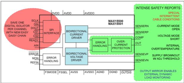
Figure 4. The MAX15500/MAX15501 output conditioner family. Device features include:  $\pm 12V$  force sense output into 1k $\Omega$ ;  $\pm 24mA$  into 750 $\Omega$ ; 100µs settling time to 14 bits; 40µs settling time to 12 bits.
