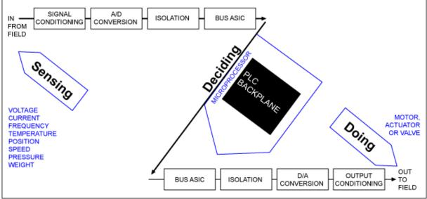
Figure 3. Simplified PLC block diagram.
