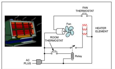
Figure 1. A household electric heater, a simple example of process control.
