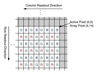
Figure 5. Pixel Color Pattern Detail RGB Bayer (Top Right Corner)
