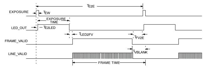
Figure 17. Snapshot Mode Frame Synchronization Waveforms
