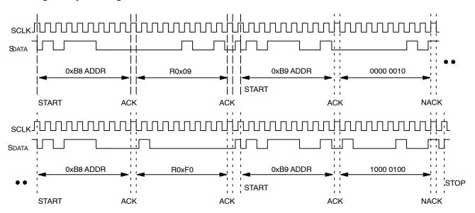
Figure 12. Timing Diagram Showing a Bytewise Read from R0x09; Returned Value 0x0284
