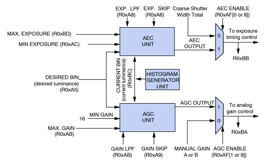
Figure 28. Controllable and Observable AEC/AGC Registers
