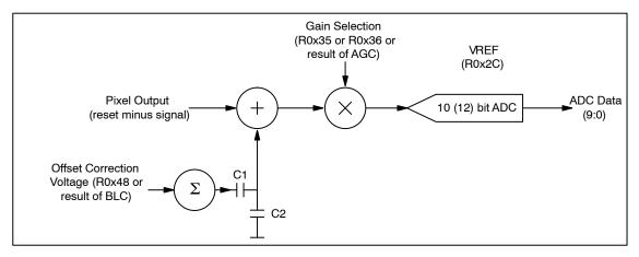
Figure 27. Black Level Calibration Flow Chart
