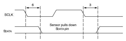
Figure 44. Acknowledge Signal Timing After an 8-Bit WRITE to the Sensor
