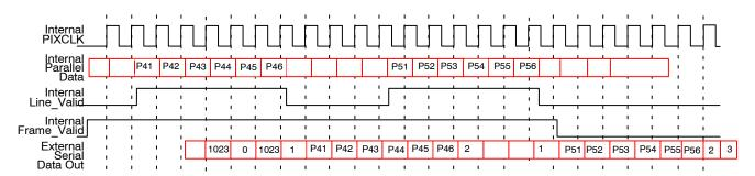
Figure 35. Serial Output Format for a 6x2 Frame
