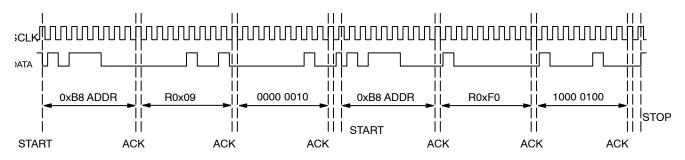
Figure 11. Timing Diagram Showing a Bytewise Write to R0x09 with the Value 0x0284
