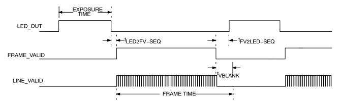
Figure 15. Sequential Master Mode Synchronization Waveforms
