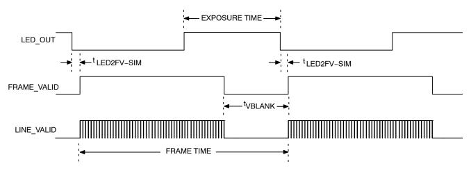
Figure 13. Simultaneous Master Mode Synchronization Waveforms #1
