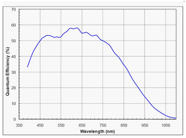
Figure 47. Typical Quantum Efficiency – Monochrome
