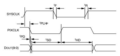
Figure 37. Propagation Delays for PIXCLK and Data Out Signals
