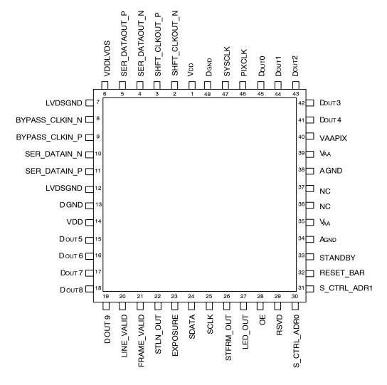
Figure 2. 48-Pin CLCC Package Pinout Diagram
