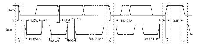
Figure 39. Two-Wire Serial Bus Timing Parameters
