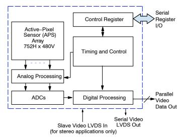
Figure 1. Block Diagram
