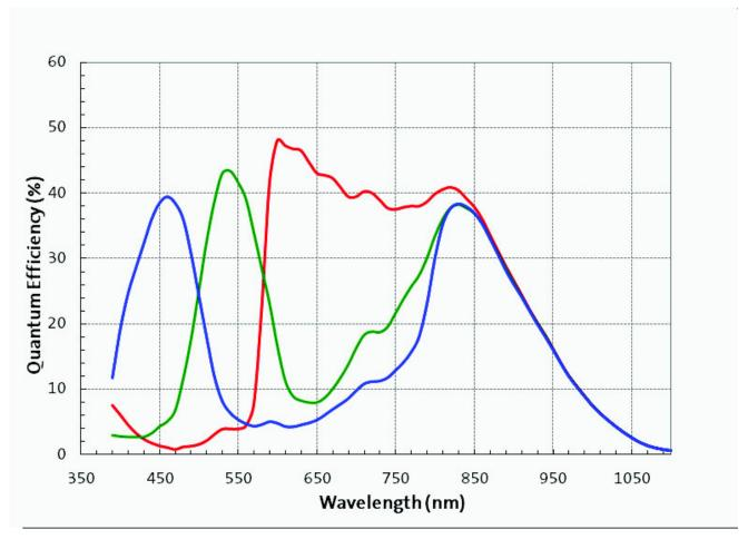
Figure 46. Typical Quantum Efficiency - RGB Bayer
