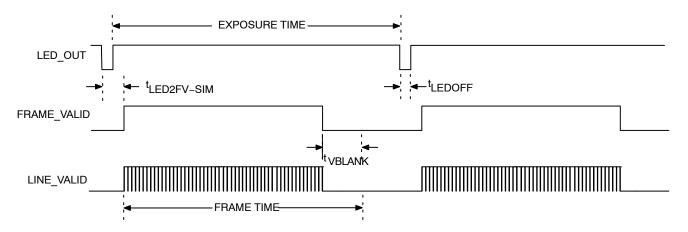
Figure 14. Simultaneous Master Mode Synchronization Waveforms #2
