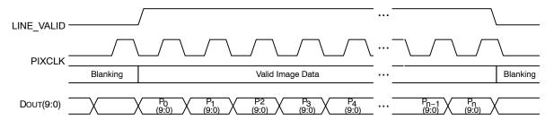
Figure 7. Timing Example of Pixel Data
