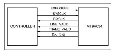
Figure 16. Snapshot Mode Interface Signals
