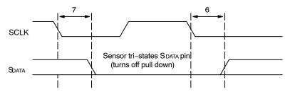
NOTE: After a READ, the master receiver must pull down SDATA to acknowledge receipt of data bits. When read sequence is complete, the master must generate a "No Acknowledge" by leaving SDATA to float HIGH. On the following cycle, a start or stop bit may be used.
