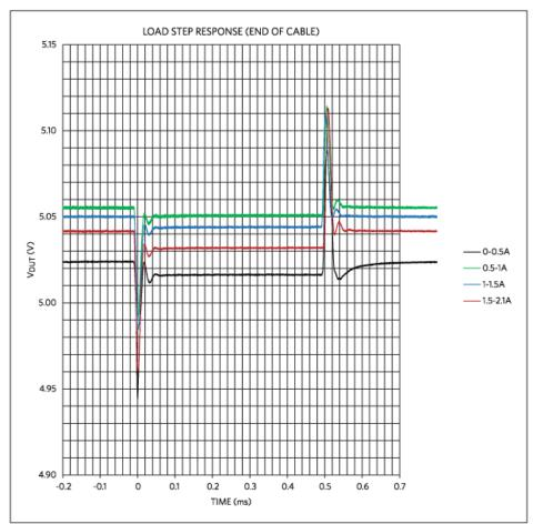
Figure 6. Data show the MAX16984 the load step response at the end of the cable. This performance prevents any overvoltage transients from reaching the PD.
