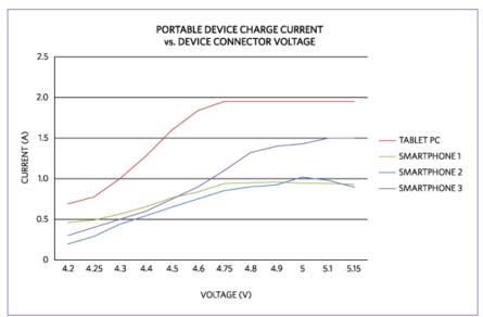
Figure 1. Four of today's leading smartphones and tablets were tested for performance. When the voltage at the PD is below the USB specification, it causes reduced charging current and a longer charge time.
