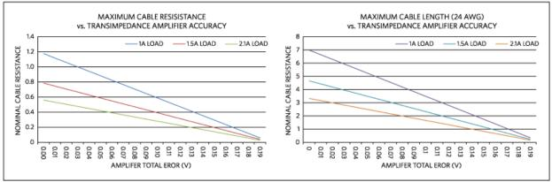
Figure 5. Nominal cable properties vs. total amplifier error.
