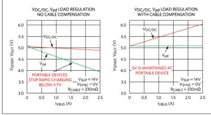
Figure 4. Data from the MAX16984 show how 5V is maintained for the PD.
