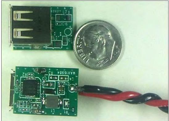
Figure 8. Form factor for complete MAX16984 solution shown next to a U.S. 10-cent coin.
