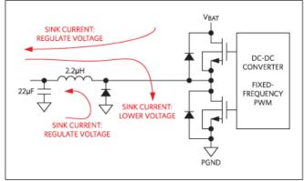
Figure 3. The MAX16984 sourcing/sinking supply.
