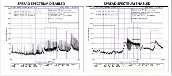
Figure 2. Spread spectrum enabled/disabled for the MAX16984.
