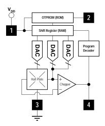
Pin 1 - V<sub>DD</sub> (Supply)
