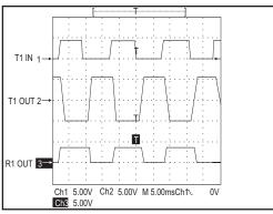
Figure 3. Loopback Test Circuit result at 120Kbps (All Drivers Fully Loaded)
