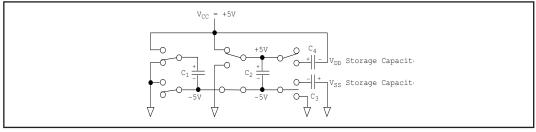
Figure 8. Charge Pump - Phase 3
