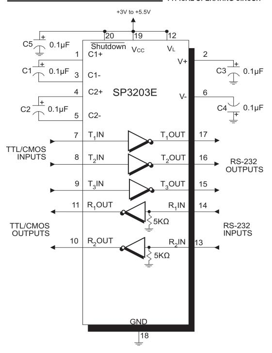
Figure 1. SP3203E Typical Operating Circuit
