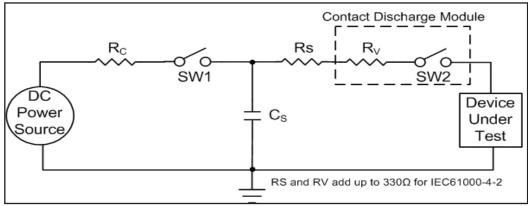
Figure 12. ESD Test Circuit for IEC61000-4-2
