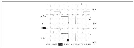
Figure 7. Charge Pump Waveforms
