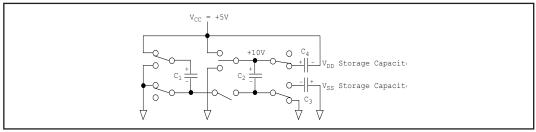
Figure 9. Charge Pump - Phase 4
