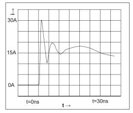
Figure 13. ESD Test Waveform for IEC61000-4-2
