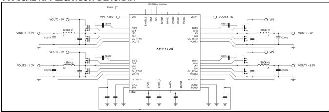
Fig. 1: XRP7724 Application Diagram
