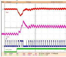
Fig. 7 0-6A Transient 300kHz PWM only
