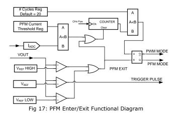
The PFM loop works in conjunction with the PWM loop and is entered when the output current falls below a programmed threshold level for a programmed number of cycles. When PFM mode is entered, the PWM loop is disabled and instead, the scaled output voltage is compared to Vref with a window comparator. The window comparator has three thresholds; normal (Vref), high (Vref + %high) and low (Vref - %low). The %high and %low values are programmable and track Vref.
