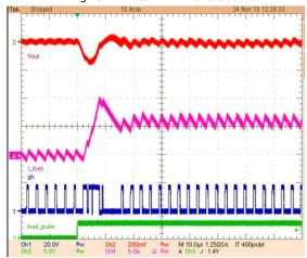
Fig. 8 10-6A Transient 300kHz with OVS  $\pm 5.5\%$
