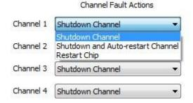
In the case of shutting down the faulting channel and auto-restarting, the user has an option to specify startup timeout (the time in which the fault is validated) and hiccup timeout (the period after which the controller will try to restart the channel) periods in 1 msec increments with a maximum value of 255 msec.
