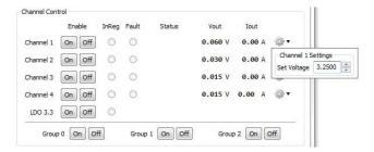
Channels including LDO3.3 can be controlled independently by any GPIO/PSIO or I2C command. Channels will start-up or shutdown following transitions of signals applied to GPIO/PSIOs set to control the channels. The control can always be overridden with an I2C command.
