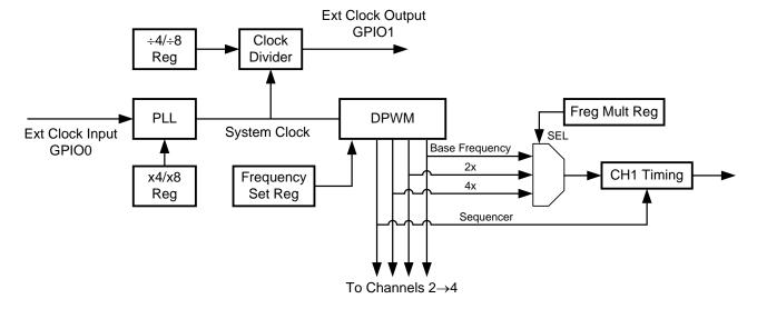
Fig 18 XRP7724 Timing Block Diagram
