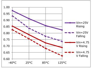
Fig. 15: Enable Threshold Over Temp
