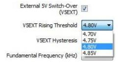
When the controller switches over to the V5EXT rail, the V5EXT\_RISE interrupt is generated to inform the host. Similarly, when the controller switches out, the V5EXT\_FALL interrupt gets generated.
