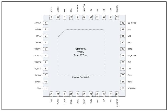
Fig. 4: XRP7724 Pin Assignment
