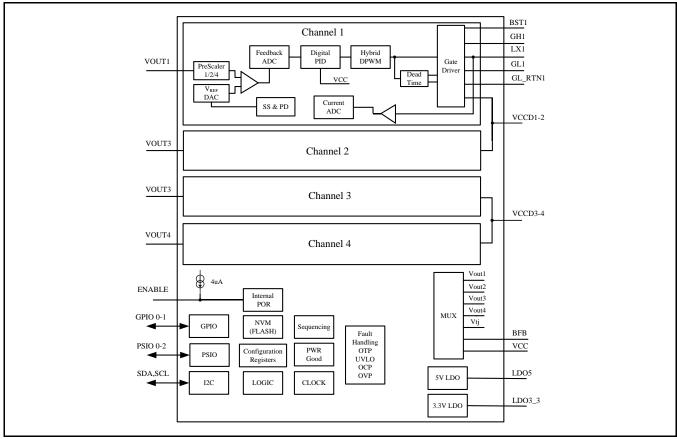
Fig. 2: XRP7724 Block Diagram
