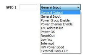
• **HW Power Good** – the Power Good hardware monitoring function. It can only be forwarded to GPIO1. It is an output voltage monitoring function that is a hardware comparison of channel output voltage against its user defined Power Good threshold limits (Power Good minimum and maximum levels). It has no hysteresis. Multiple channel selection is available in which case the resulting signal is the AND logic function of all channels selected.
