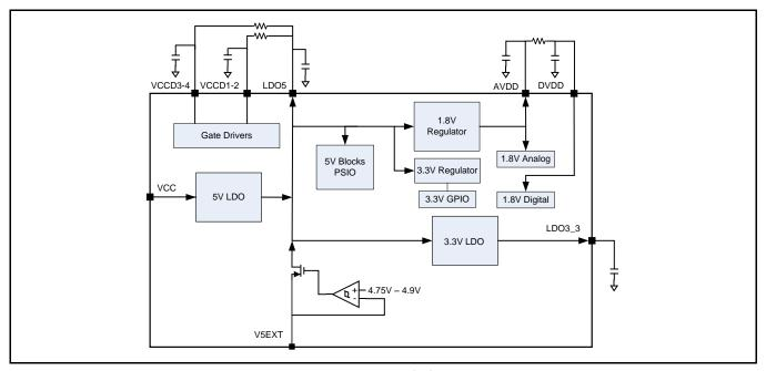
Fig. 3: XRP7724 LDO Block Diagram
