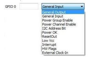
**HW Flags** – these are hardware monitoring functions forwarded to GPIO0 only. The functions include Under-Voltage Warning, Over- Temperature Warning, Over-Voltage Fault, Over-Current Fault and Over -Current Warning for every channel. Multiple selection is available in which case the resulting signal is the OR logic function
