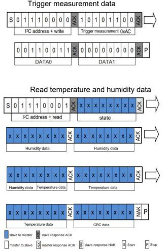
Note: The sensor needs time to collect. After the host sends a measurement command (0xAC), delay more than 80 milliseconds before reading the converted data and judging whether the returned status bit is normal. If the status bit [Bit7] is 0, it means that the data can be read normally. When it is 1, the sensor is busy, and the host needs to wait for the data processing to complete.
