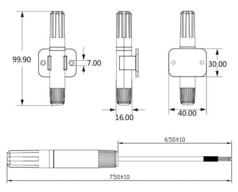
Figure 12. AM2315C sensor encapsulation (unit: mm not specified tolerance: ± 0.2 mm)
