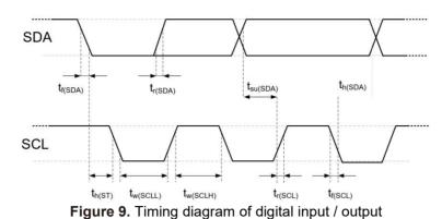
The abbreviations are explained in Table 7. The thicker SDA line is controlled by the sensor, and the ordinary SDA line is controlled by the single-chip microcomputer. Please note that the SDA valid read time is triggered by the falling edge of the previous conversion.
