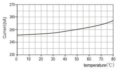
**Figure 6.** Typical supply current vs. temperature curve (sleep mode) when VDD=3.3V Please note: There is a deviation of approximately ±25% between these data and the displayed value.
