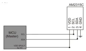
Figure 8. Typical application circuit
