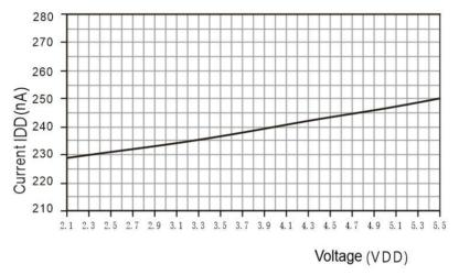
**Figure 7.** The relationship between current and voltage at  $25^{\circ}$ C
