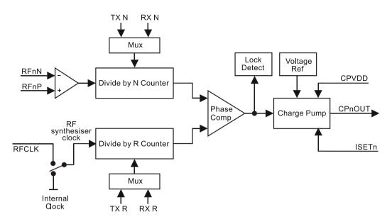
Figure 17 Single RF PLL Block Diagram
