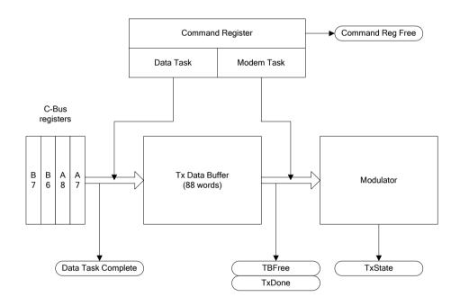
Figure 11 Tx Task Operation
