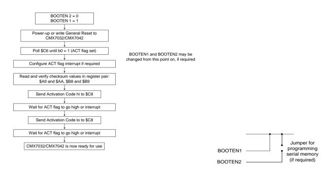
Figure 8 FI Loading from Serial Memory
