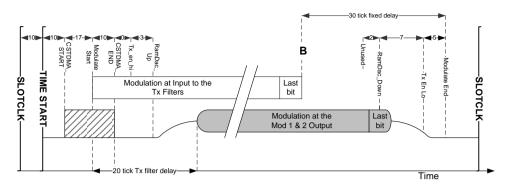
Figure 13 Typical AIS Transmission
