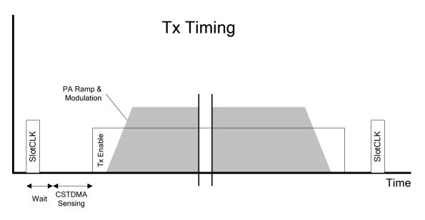
Figure 9 Tx Burst Timing
