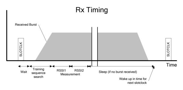
Figure 10 Rx Burst Timing
