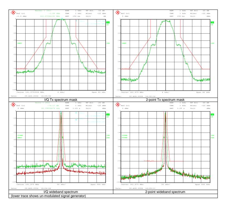
Figure 14 Tx Spectrum Masks
