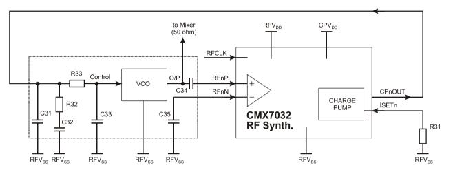
Figure 16 Example RF Synthesiser Components
