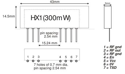
Figure 3: HX1 pin-out and dimension
