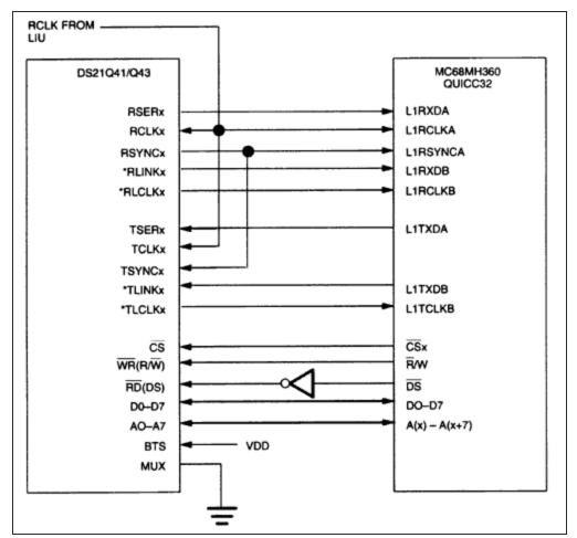
Figure 1. Quad framer - QUICC32 interconnections.
