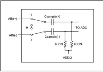
Figure 1. Fully-differential T/H stage.
