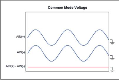
Figure 9. Common-mode voltage.
