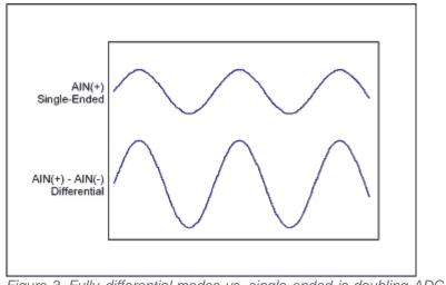
Figure 3. Fully-differential modes vs. single-ended is doubling ADC dynamic range.
