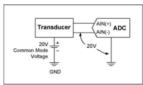
Figure 4. High common-mode voltage.
