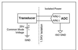
Figure 5. High common-mode voltage with a separate system power supply.
