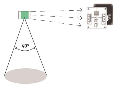
Fig. 4 Diagram of the MR24BSD1 radar coverage area Due to the radar beam characteristics, the radar has a relatively long range
