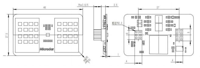
Fig. 1 Schematic diagram of the radar module structure
