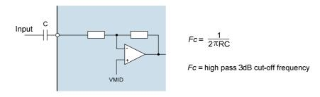
Figure 9 Audio Input Path DC Blocking Capacitor
