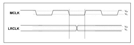
Figure 4 Recommended LRCLK Transition Area for Optimum Performance
