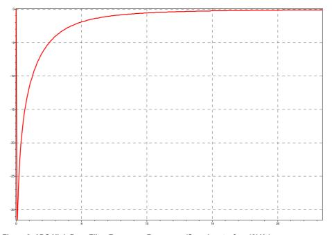
Figure 8 ADC High Pass Filter Frequency Response (Sample rate, fs = 48kHz)
