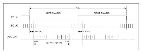
Figure 5 I<sup>2</sup>S Digital Audio Interface format (assuming n-bit word length)
