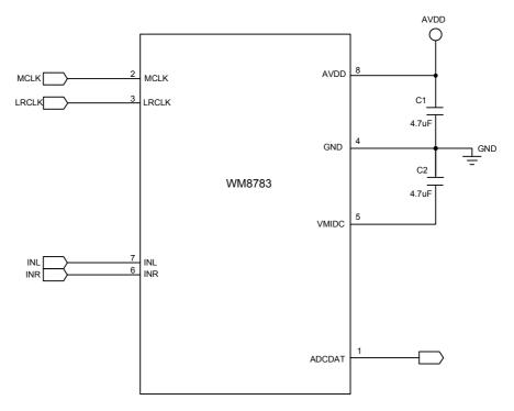
Figure 10 WM8783 Recommended External Components Diagram
