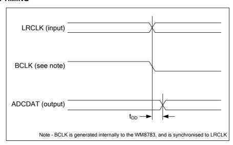
Figure 3 Audio Interface Timing
