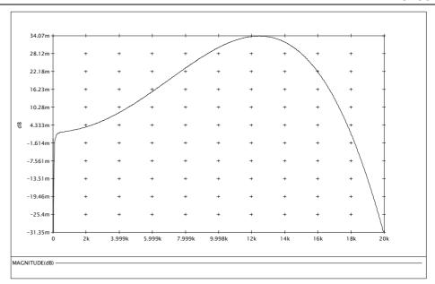
Figure 7 ADC Pass Band Frequency Response up to fs/2 (Sample rate, fs = 48kHz)
