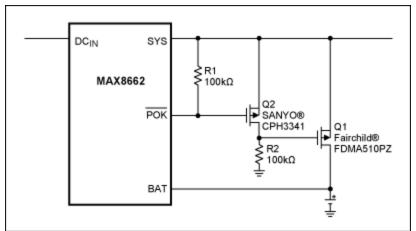
Figure 1. Simplified schematic: reducing I<sup>2</sup>R losses in Smart Power Selector-based battery chargers.
