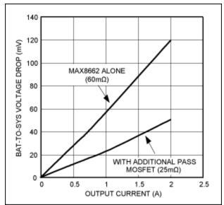
Figure 4. Data for the V<sub>BATT</sub>-to-SYS voltage vs. load current.
