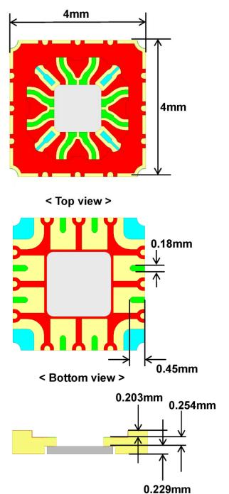
Fig. 4. CQFN 24-Pin Package Drawing (All Dimensions in mm)
