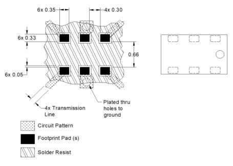
Dimensions are in Millimeters Mounting Footprint
