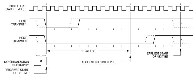
Figure 15-2. BDC Host-to-Target Serial Bit Timing
