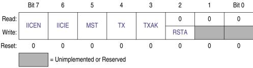
Figure 13-7. IIC Control Register (IIC1C)
