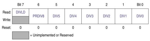
Figure 4-4. FLASH Clock Divider Register (FCDIV)
