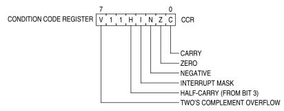
Figure 8-2. Condition Code Register
