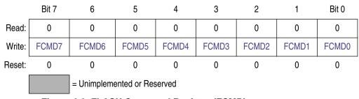
Figure 4-9. FLASH Command Register (FCMD)
