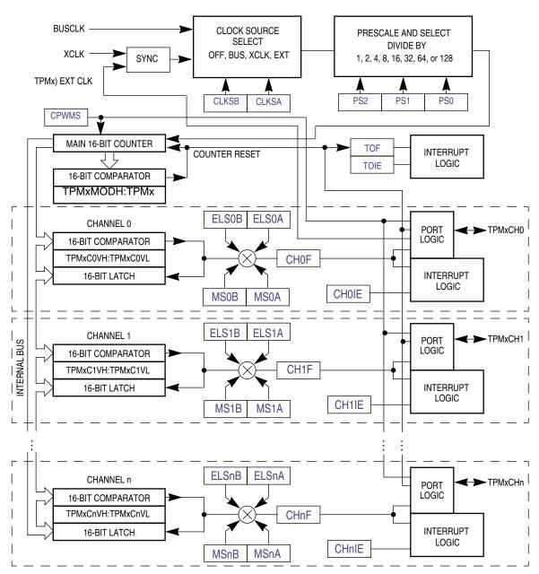
Figure 10-2. TPM Block Diagram
