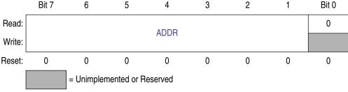
Figure 13-5. IIC Address Register (IIC1A)
