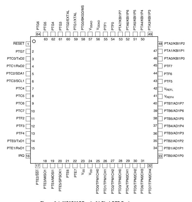
Figure 2-1. MC9S08GBxx in 64-Pin LQFP Package
