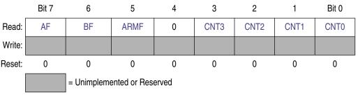
Figure 15-9. Debug Status Register (DBGS)
