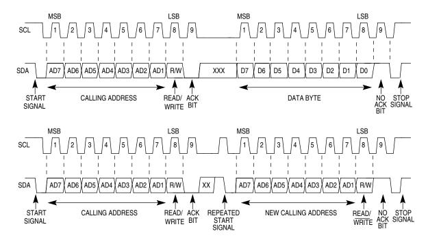
Figure 13-3. IIC Bus Transmission Signals
