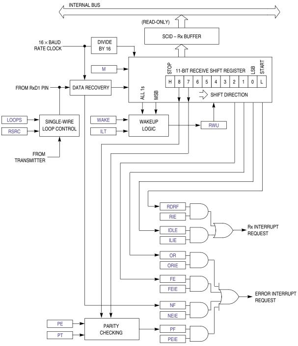
Figure 11-4. SCI Receiver Block Diagram
