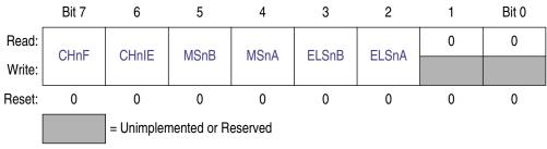
Figure 10-10. Timer x Channel n Status and Control Register (TPMxCnSC)
