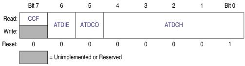
Figure 14-8. ATD Status and Control Register (ATD1SC)
