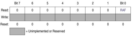
Figure 11-10. SCI x Status Register 2 (SCIxS2)
