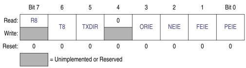
Figure 11-11. SCI x Control Register 3 (SCIxC3)
