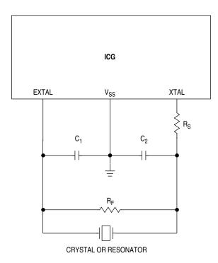
Figure 7-5. External Frequency Reference Connection
