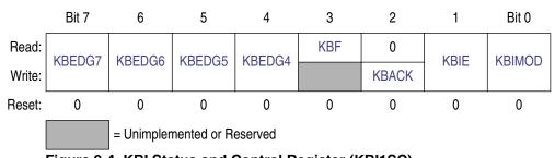
Figure 9-4. KBI Status and Control Register (KBI1SC)
