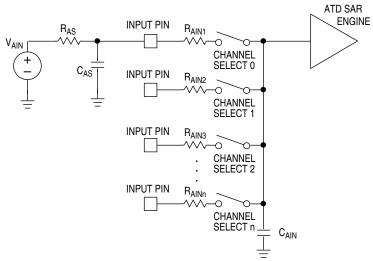
Figure 14-3. Resistor and Capacitor Placement
