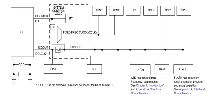
Figure 7-1. System Clock Distribution Diagram
