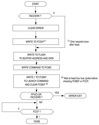
Figure 4-2. FLASH Program and Erase Flowchart
