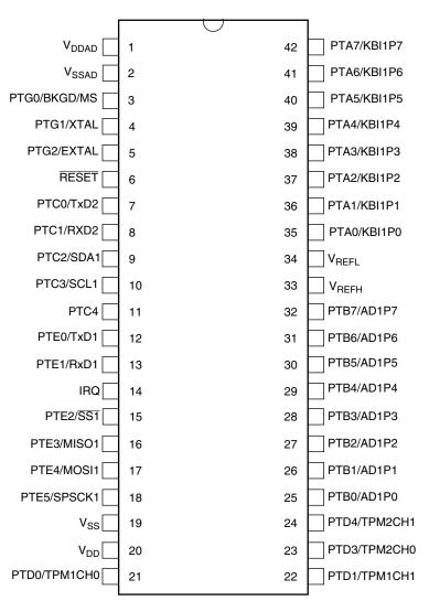
Figure 2-4. MC9S08GTxx in 42-Pin SDIP Package
