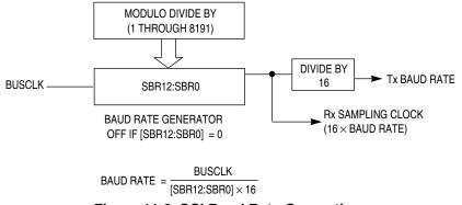
Figure 11-2. SCI Baud Rate Generation
