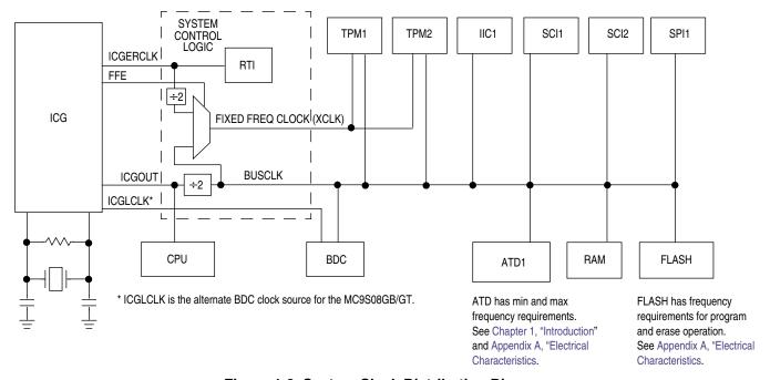
Figure 1-3. System Clock Distribution Diagram
