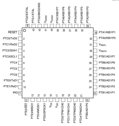
Figure 2-3. MC9S08GTxx in 44-Pin QFP Package
