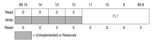
Figure 7-17. ICG Upper Filter Register (ICGFLTU)
