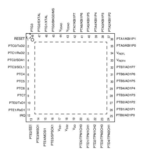
Figure 2-2. MC9S08GTxx in 48-Pin QFN Package
