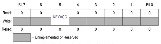
Figure 4-6. FLASH Configuration Register (FCNFG)
