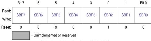
Figure 11-6. SCI x Baud Rate Register (SCIxBDL)
