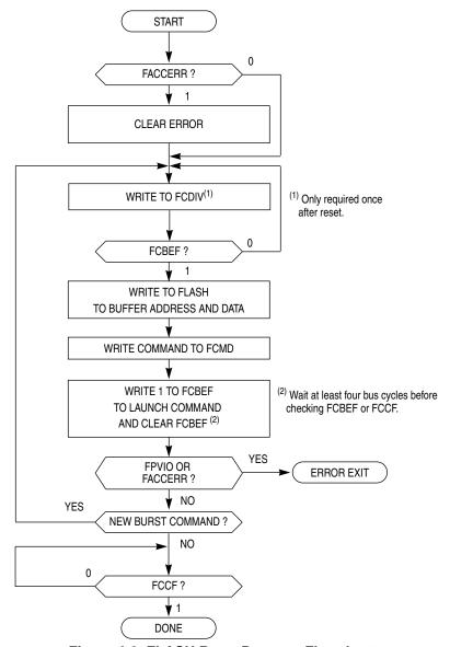
Figure 4-3. FLASH Burst Program Flowchart
