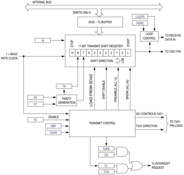
Figure 11-3. SCI Transmitter Block Diagram
