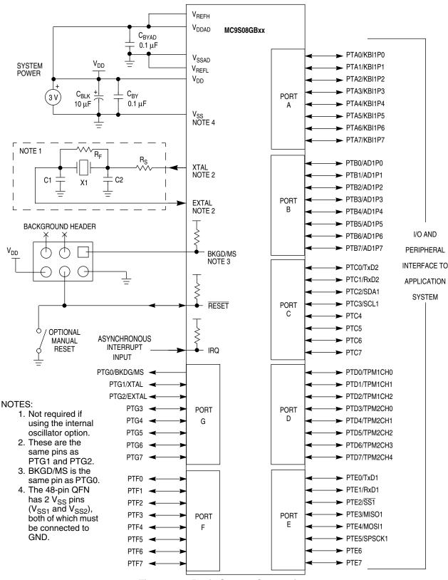
Figure 2-5. Basic System Connections
