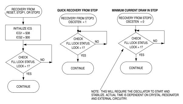
Figure 7-8. ICG Initialization for FEE in Example #1
