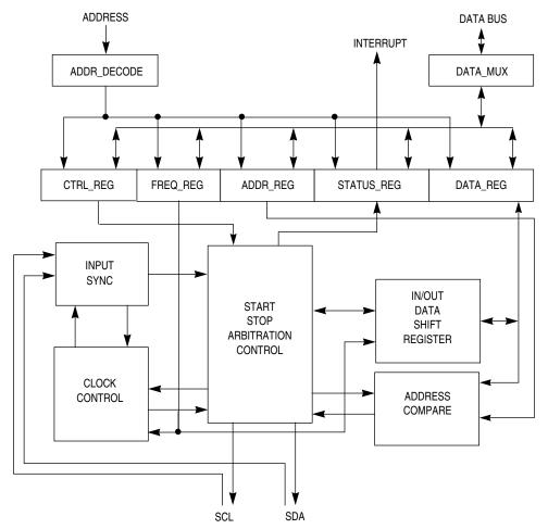
Figure 13-2. IIC Functional Block Diagram
