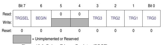
Figure 15-8. Debug Trigger Register (DBGT)
