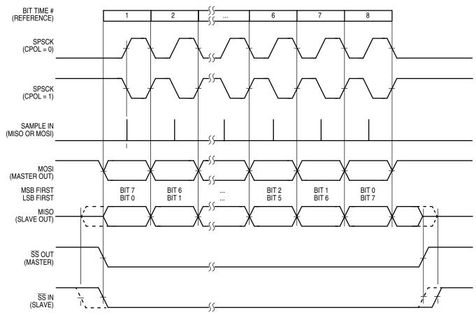
Figure 12-6. SPI Clock Formats (CPHA = 0)
