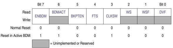
Figure 15-5. BDC Status and Control Register (BDCSCR)
