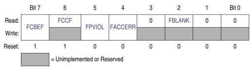
Figure 4-8. FLASH Status Register (FSTAT)
