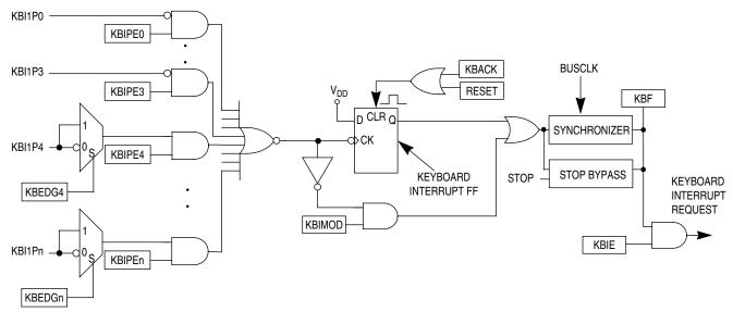
Figure 9-3. KBI Block Diagram
