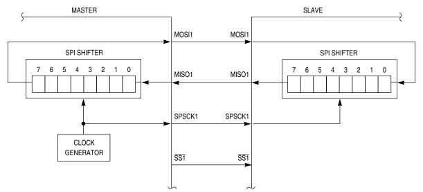
Figure 12-2. SPI System Connections
