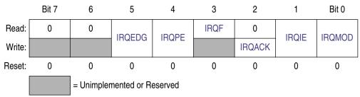
Figure 5-2. Interrupt Request Status and Control Register (IRQSC)
