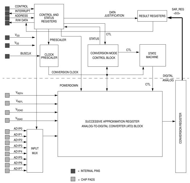
Figure 14-2. ATD Block Diagram
