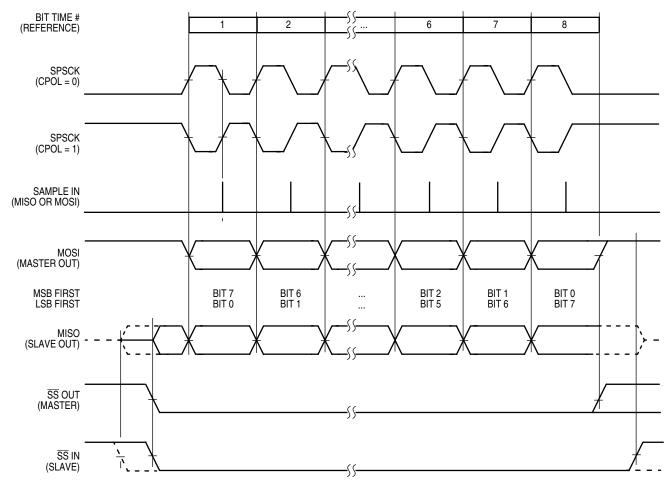
Figure 12-5. SPI Clock Formats (CPHA = 1)
