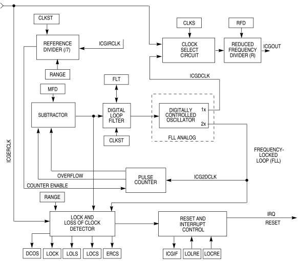
Figure 7-6. Detailed Frequency-Locked Loop Block Diagram
