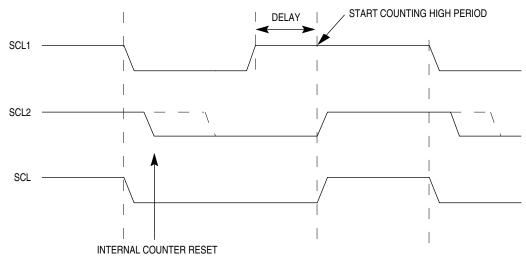
Figure 13-4. IIC Clock Synchronization
