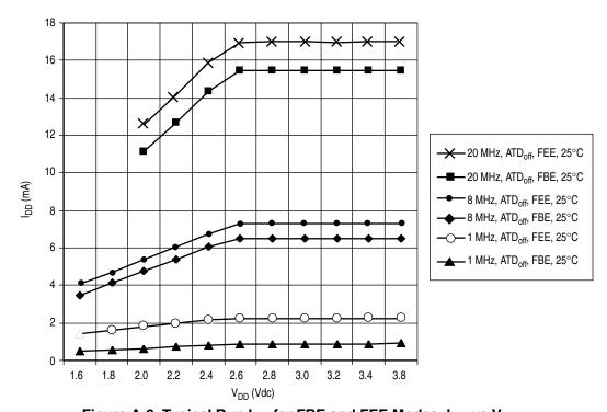
Figure A-6. Typical Run  $\rm I_{DD}$  for FBE and FEE Modes,  $\rm I_{DD}$  vs  $\rm V_{DD}$
