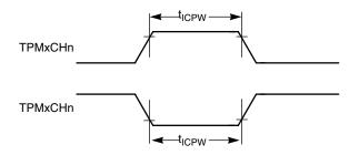
Figure A-15. Timer Input Capture Pulse
