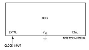
Figure 7-4. External Clock Connections
