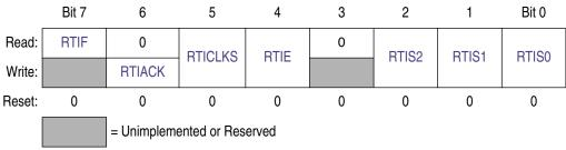
Figure 5-7. System RTI Status and Control Register (SRTISC)
