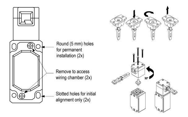
The mounting holes in the switch body accept M5 (#10) screws. There are four holes on a standard limit switch mounting pattern of 30 × 60 millimeters. The two mounting holes on the actuator are spaced 20 millimeters apart. The grommet and sleeve design allows a small amount of movement (i.e., misalignment) when the actuator engages the switch body. The sleeves accept M4.5 (#8) screws.
