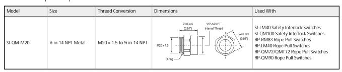
One conduit adapter is supplied with each switch.
