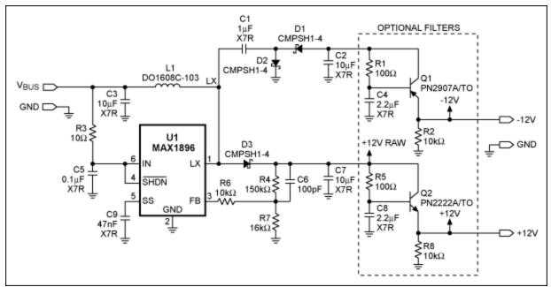
Figure 1. Powered only by a USB port, this  $\pm$ 12V supply delivers 50mA from both outputs with reasonable output regulation.
