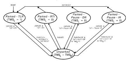
FIGURE 4. Local SCANPSC110F Bridge Port Configuration State Machine
