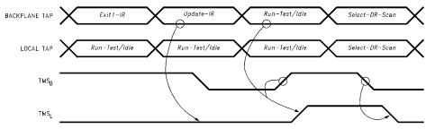
FIGURE 10. Local Scan Port Synchronization from Parked-RTI State
