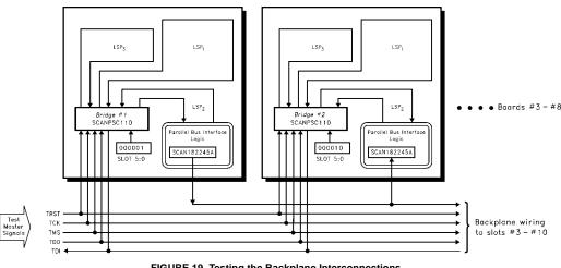
FIGURE 19. Testing the Backplane Interconnections
