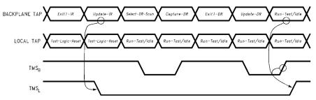
FIGURE 11. Local Scan Port Synchronization on Second Pass
