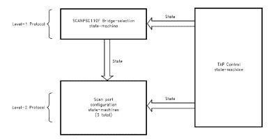
FIGURE 2. SCANPSC110F Bridge State Machines
