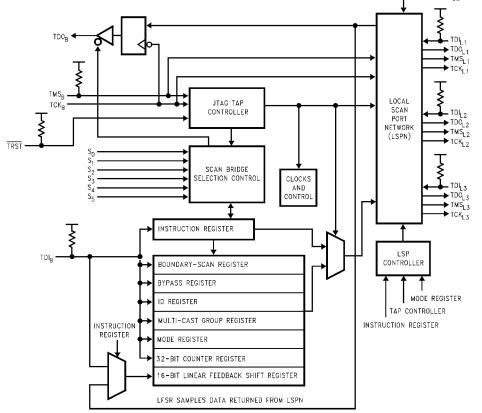
FIGURE 1. SCANPSC110F Bridge Architecture
