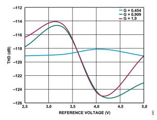
Figure 21. THD vs. Reference Voltage, G = 0.454, G = 0.909, and G = 1.9,  $f_{IN} = 1 \text{ kHz}$
