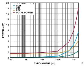
Figure 32. Power vs. Throughput
