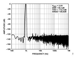
Figure 15. 1 kHz, -0.5 dBFS Input Tone FFT, Wide View, G = 1, V<sub>REF</sub> = 2.5 V, Single-Ended
