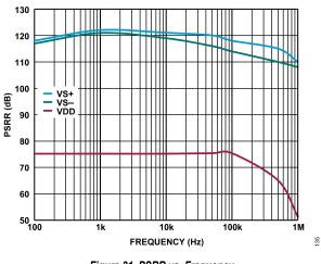
Figure 31. PSRR vs. Frequency
