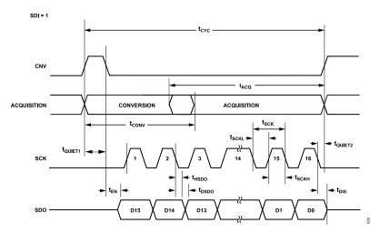
Figure 57. 3-Wire CS Turbo Mode Serial Interface Timing Diagram (SDI High)
