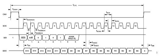
Figure 52. Register Read Timing Diagram
