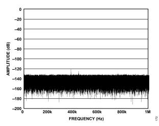
Figure 70. FFT with Shorted Inputs
