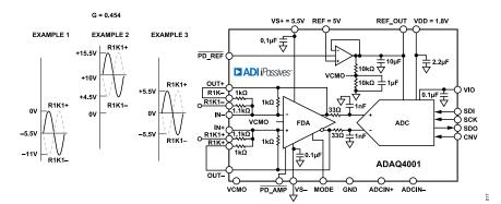
Figure 45. Differential Configuration with G = 0.454
