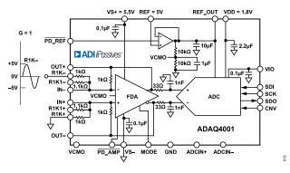
Figure 43. Single-Ended to Differential Configuration with G = 1
