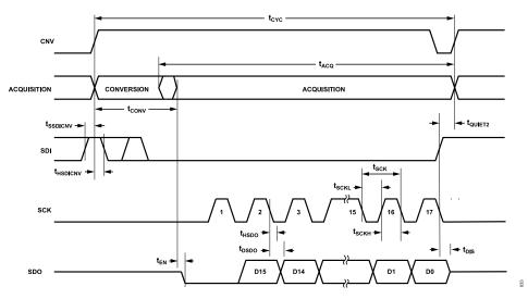
Figure 67. 4-Wire CS Mode with the Busy Indicator Serial Interface Timing Diagram
