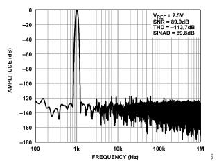
Figure 16. 1 kHz, -0.5 dBFS Input Tone FFT, Wide View, Differential, G = 0.909, V<sub>REF</sub> = 2.5 V, Low Power Mode
