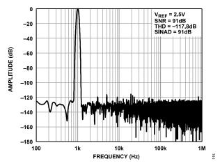
Figure 14. 1 kHz, -0.5 dBFS Input Tone FFT, Wide View, G = 1, V<sub>REF</sub> = 2.5 V, Differential
