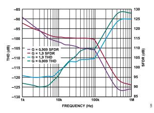
Figure 27. THD and SFDR vs. Frequency for G = 0.909 and G = 1.9, V<sub>REF</sub> = 5 V
