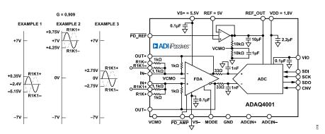
Figure 46. Differential Configuration with G = 0.909
