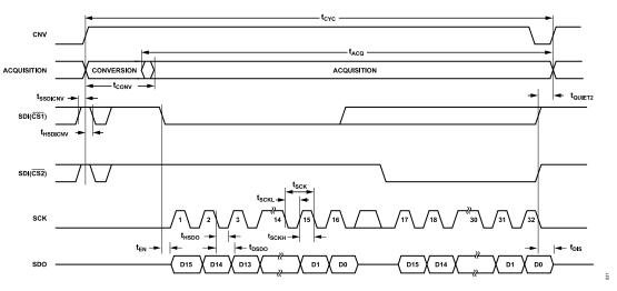
Figure 65. 4-Wire CS Mode Without the Busy Indicator Serial Interface Timing Diagram
