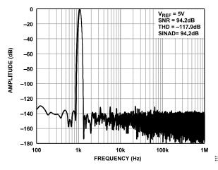
Figure 13. 1 kHz, -0.5 dBFS Input Tone FFT, Wide View, Differential, G = 0.909, V<sub>REF</sub> = 5 V, Low Power Mode
