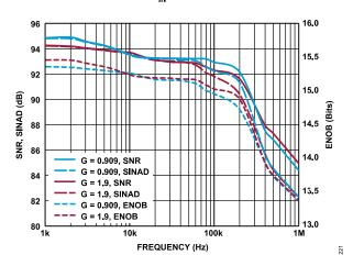
Figure 24. SNR, SINAD, and ENOB vs. Frequency for G = 1.9 and G = 0.909,  $V_{REF}$  = 5 V
