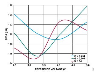
Figure 22. SFDR vs. Reference Voltage for G = 0.454, G = 0.909, and G = 1.9,  $f_{IN} = 1 \text{ kHz}$
