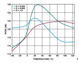
Figure 26. SFDR vs. Temperature for G = 0.454, G = 0.909, and G = 1.9,  $f_{\rm IN}$  = 1kHz
