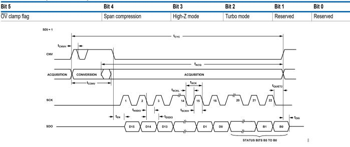
Figure 55. 3-Wire CS Mode Without the Busy Indicator, Including Status Bits, Serial Interface Timing Diagram (SDI High)
