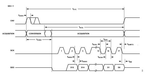
Figure 61. 3-Wire CS Mode with the Busy Indicator Serial Interface Timing Diagram (SDI High)
