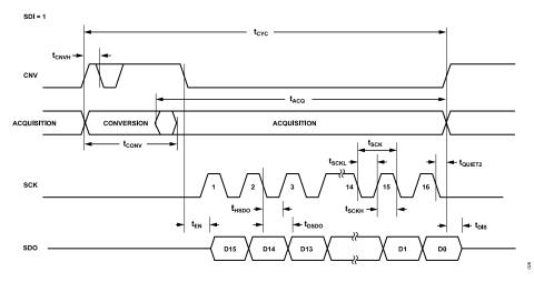
Figure 59. 3-Wire CS Mode Without the Busy Indicator Serial Interface Timing Diagram (SDI High)
