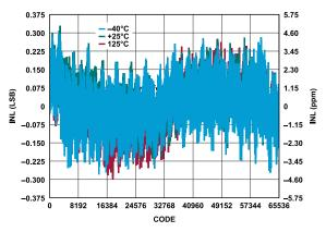
Figure 5. INL vs. Code for Various Temperatures, V<sub>REF</sub> = 5 V, G = 0.454
