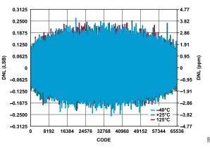
Figure 8. DNL vs. Code for Various Temperatures, V<sub>REF</sub> = 5 V, G = 0.454
