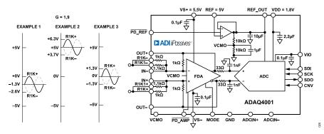
Figure 48. Differential Configuration with G = 1.9
