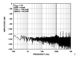
Figure 17. 100 kHz, -0.5 dBFS Input Tone FFT, Wide View, G = 1, V<sub>REF</sub> = 5 V
