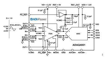
Figure 44. Single-Ended to Differential Configuration with G = 1.9
