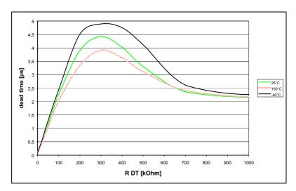
Fig. 9: Typ. dead time internal generated
