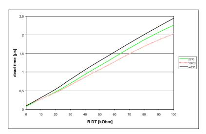
Fig. 10: Typ. dead time internal generated - detail
