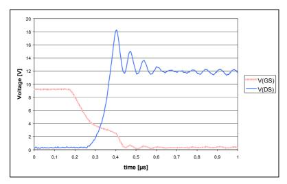
Fig. 17: typ. fall-time at 25°C
