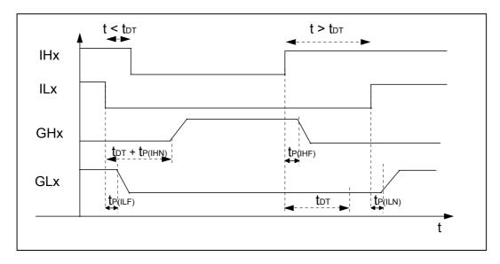
Fig. 7: Dead time generation when IHx and ILx are seperated
