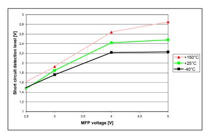
Fig. 15: Short circuit detection level
