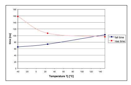
Fig. 19: Rise- and fall-times vs. temperature  $T_{\rm J}$
