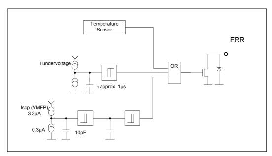
Fig. 5: Block diagram of ERR functionality
