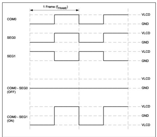
Figure 2. Alternating drive waveforms for static LCD segments.
