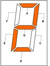
Figure 1. Seven-segment LCD display digit.
