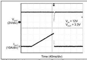
FIGURE 2-69: Output Peak Current-Limit Threshold.
