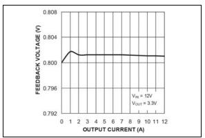
**FIGURE 2-12:** Feedback Voltage vs. Output Current (MIC2101).
