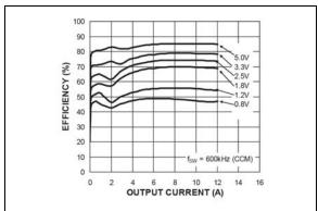
**FIGURE 2-18:** Efficiency  $(V_{IN} = 38V)$  vs. Output Current (MIC2101).
