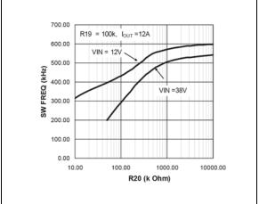
FIGURE 5-2: Switching Frequency vs. R20.
