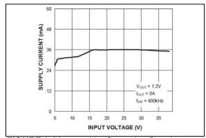
FIGURE 2-23: V<sub>IN</sub> Operating Supply Current vs. Input Voltage (MIC2102).
