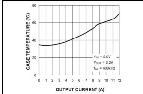
**FIGURE 2-36:** Case Temperature\*  $(V_{IN} = 5.0V)$  vs. Output Current.
