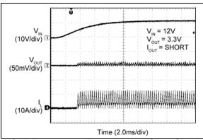
FIGURE 2-65: Power-Up into Short Circuit.
