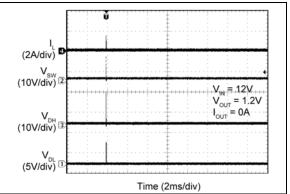
**FIGURE 2-88:** MIC2101 Switching Waveforms ( $I_{OUT} = 0A$ ).
