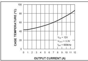
**FIGURE 2-37:** Case Temperature\*  $(V_{IN} = 12V)$  vs. Output Current.
