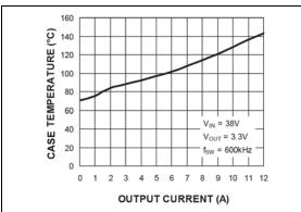
**FIGURE 2-39:** Case Temperature\*  $(V_{IN} = 38V)$  vs. Output Current.
