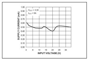
**FIGURE 2-1:** V<sub>IN</sub> Operating Supply Current vs. Input Voltage (MIC2101).
