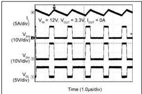
**FIGURE 2-78:** MIC2102 Switching Waveforms ( $I_{OUT} = 0A$ ).
