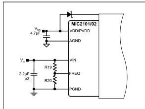
FIGURE 5-1: Switching Frequency Adjustment.
