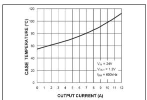
**FIGURE 2-42:** Case Temperature\*  $(V_{IN} = 24V)$  vs. Output Current.
