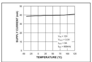
**FIGURE 2-24:** V<sub>IN</sub> Operating Supply Current vs. Temperature (MIC2102).
