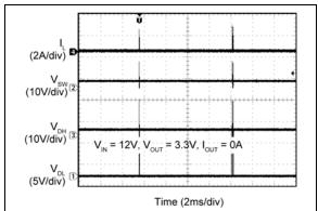
**FIGURE 2-76:** MIC2101 Switching Waveforms ( $I_{OUT} = 0A$ ).
