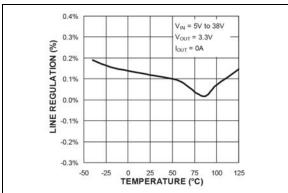
FIGURE 2-27: Line Regulation vs. Temperature (MIC2102).
