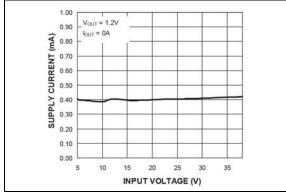
**FIGURE 2-3:** V<sub>IN</sub> Operating Supply Current vs. Input Voltage (MIC2101).
