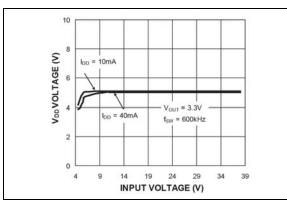
**FIGURE 2-45:** V<sub>DD</sub> Voltage vs. Input Voltage.
