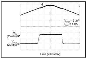
FIGURE 2-64: V<sub>IN</sub> UVLO Thresholds.
