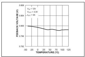
**FIGURE 2-9:** Feedback Voltage vs. Temperature (MIC2101).
