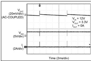
**FIGURE 2-74:** MIC2101 Switching Waveforms ( $I_{OUT} = 0A$ ).
