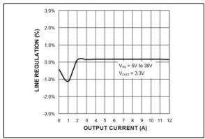
**FIGURE 2-13:** Line Regulation vs. Output Current (MIC2101).
