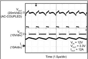
**FIGURE 2-71:** MIC2102 Switching Waveforms ( $I_{OUT} = 12A$ ).
