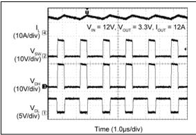
**FIGURE 2-75:** MIC2101 Switching Waveforms ( $I_{OUT} = 12A$ ).
