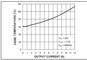
**FIGURE 2-38:** Case Temperature\*  $(V_{IN} = 24V)$  vs. Output Current.
