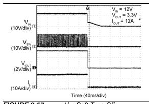
FIGURE 2-57: V<sub>IN</sub> Soft Turn-Off.
