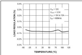
FIGURE 2-26: Load Regulation vs. Temperature (MIC2102).
