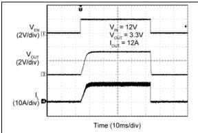
FIGURE 2-62: Enable Turn-On/Turn-Off.
