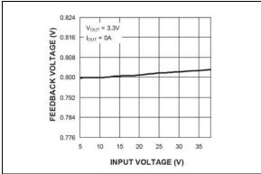
FIGURE 2-5: Feedback Voltage vs. Input Voltage (MIC2101).
