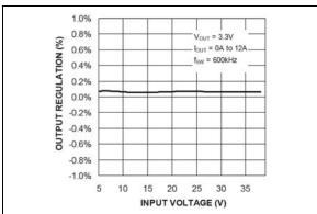
FIGURE 2-21: Output Regulation vs. Input Voltage (MIC2102).
