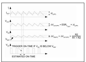
FIGURE 4-1: MIC2101/2 Control Loop Timing.
