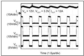
**FIGURE 2-77:** MIC2102 Switching Waveforms ( $I_{OUT} = 12A$ ).
