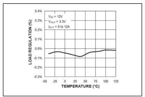
FIGURE 2-10: Load Regulation vs. Temperature (MIC2101).
