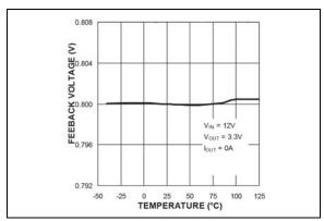
**FIGURE 2-25:** Feedback Voltage vs. Temperature (MIC2102).
