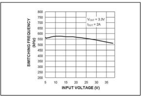
FIGURE 2-47: Switching Frequency vs. Input Voltage.
