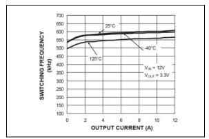
**FIGURE 2-28:** Switching Frequency vs. Output Current (MIC2102).
