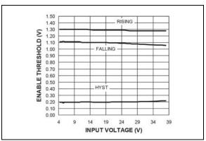
FIGURE 2-46: Enable Threshold vs. Input Voltage.
