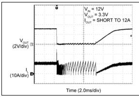
FIGURE 2-68: Output Recovery from Short Circuit.
