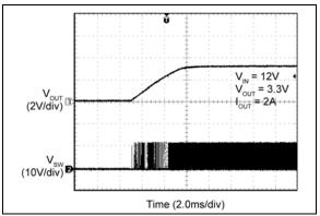
**FIGURE 2-70:** Output Recovery from Thermal Shutdown.
