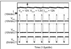
**FIGURE 2-87:** MIC2101 Switching Waveforms ( $I_{OUT} = 12A$ ).
