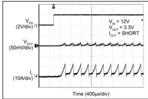
FIGURE 2-66: Enabled into Short.
