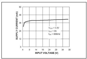
**FIGURE 2-19:** V<sub>IN</sub> Operating Supply Current vs. Input Voltage (MIC2102).
