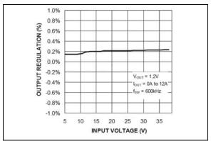
**FIGURE 2-22:** Output Regulation vs. Input Voltage (MIC2102).
