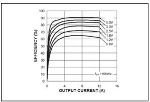
**FIGURE 2-34:** Efficiency  $(V_{IN} = 24V)$  vs. Output Current (MIC2102).
