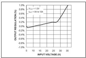
FIGURE 2-4: Output Regulation vs. Input Voltage (MIC2101).
