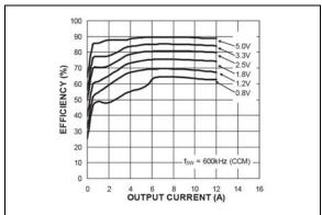
**FIGURE 2-17:** Efficiency  $(V_{IN} = 24)$  vs. Output Current (MIC2101).
