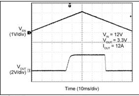
FIGURE 2-63: Enable Thresholds.
