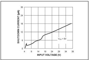
**FIGURE 2-44:** V<sub>IN</sub> Shutdown Current vs. Input Voltage.
