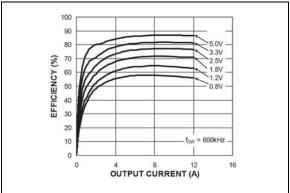
**FIGURE 2-35:** Efficiency  $(V_{IN} = 38V)$  vs. Output Current (MIC2102).
