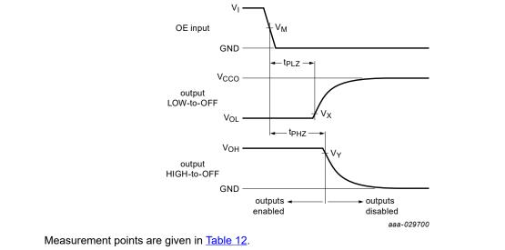
V<sub>OL</sub> and V<sub>OH</sub> are typical output voltage levels that occur with the output load.
