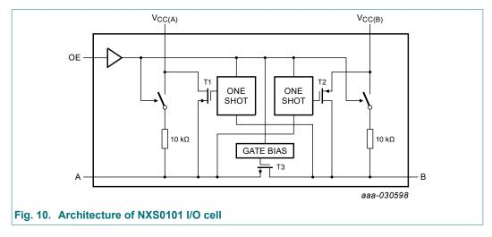
The NXS0101 is a "switch" type voltage translator, it employs two key circuits to enable voltage translation:
