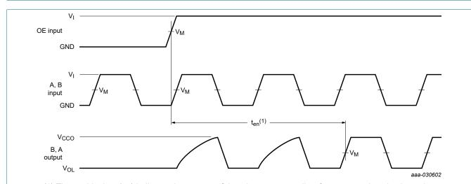
(1) The enable time  $(t_{en})$  indicates the amount of time the user must allow for one one-shot circuitry to become operational after OE is taken HIGH. See also Section 13.6.
